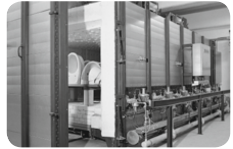
Intermittent shuttle kiln in the ceramics industry
