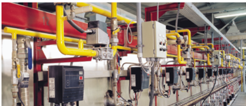
Roller hearth kiln in the ceramics industry
