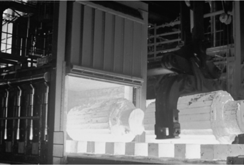
Bogie hearth forging furnace in the metallurgical industry
